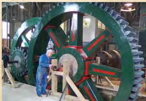
Left: Merv Grafton from the Bella Street Pumphouse Society oils the bearings of the replica flywheel the Society built to demonstrate the scale of the heavy engineering.
